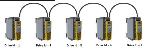
Each drive owns its own Id (1 to 5, Application::PTP::Drive Id), and should contain this control diagram in its application.
