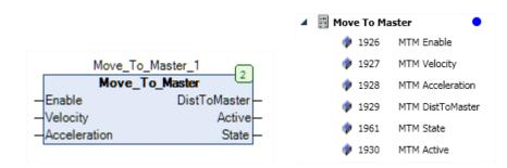
When *Enable*, if an offset exists when the Slave drive is enabled, the Slave will move to the Master position in a controlled movement.
